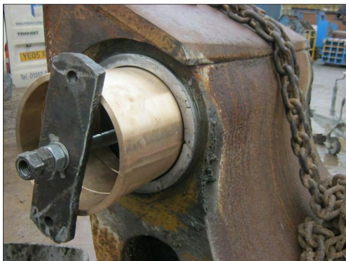
New jaw stock hinge pin bush being fitted.
