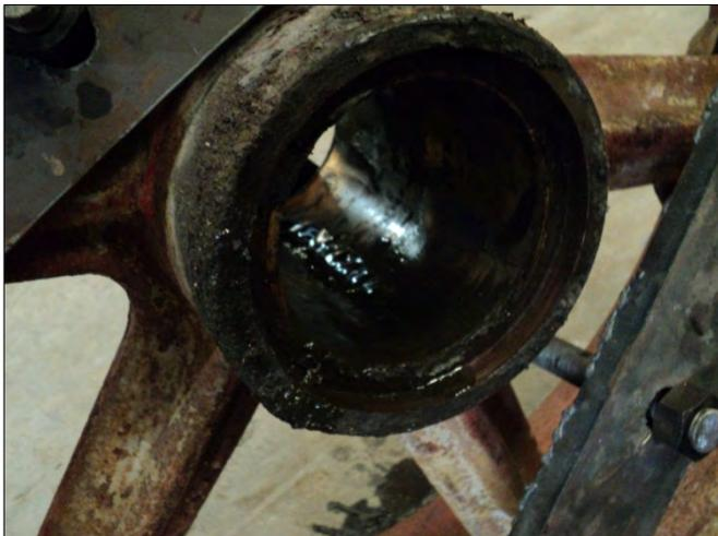
After removing fly wheel bronze bush was found to be worn out.
