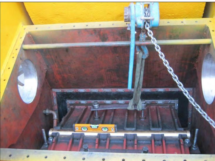
Pitman toggles and toggle pin fitted.
