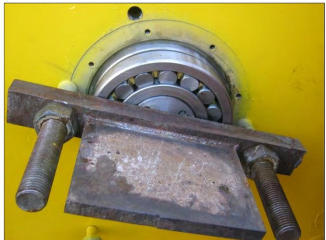
Pressing bearings into main frame.
