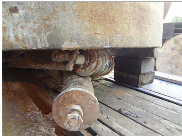
Damaged draw back bolts that we replaced.
