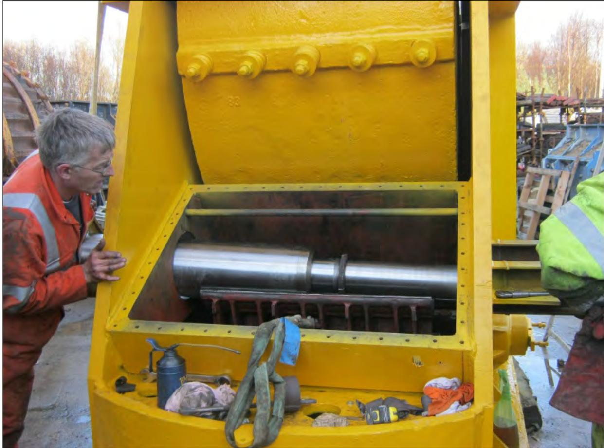
*Eccentric shaft and bearing assembly being fitted*
