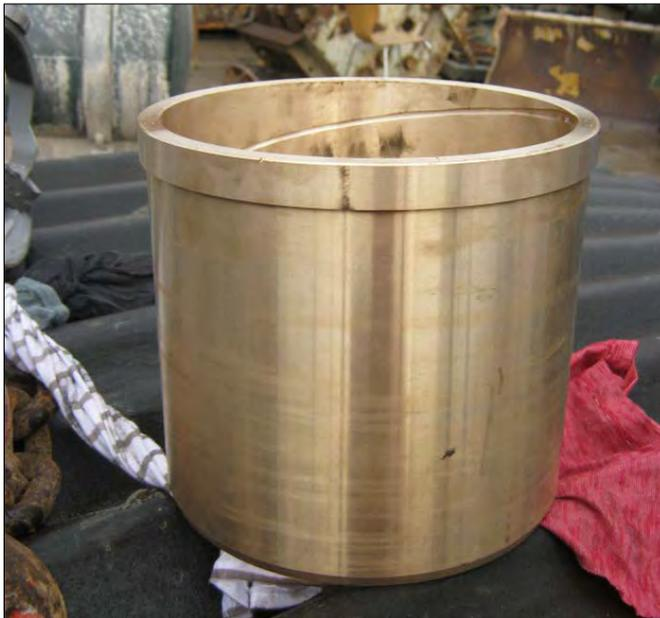
New hinge pin bushes to be fitted to both sides of jaw stock.
