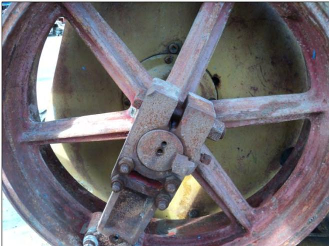
Flywheel to be removed due oscillation movement.
