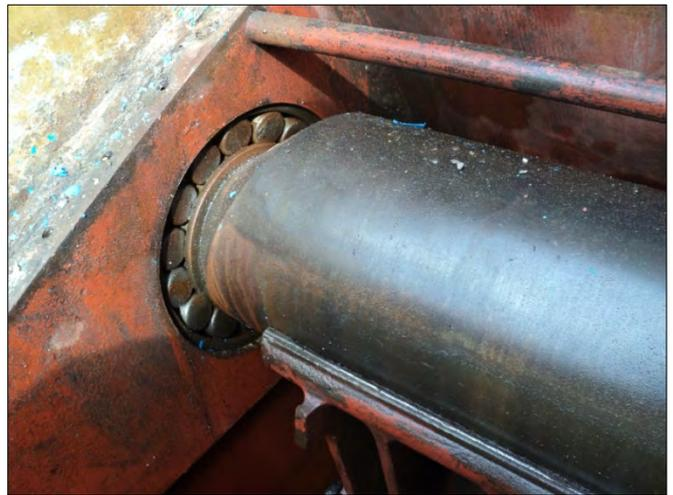
Bearings rusted and in poor condition due to lack of lubrication.
