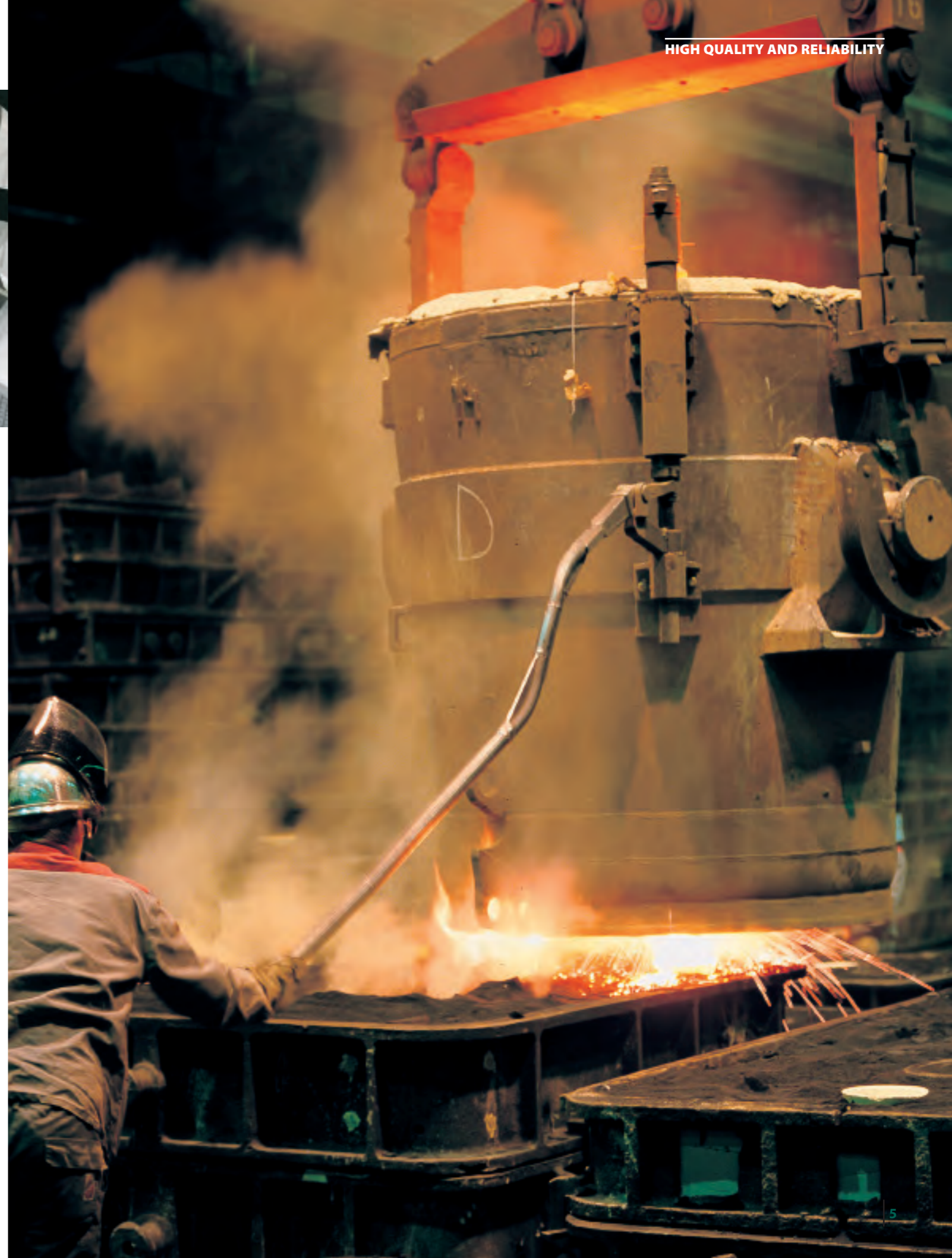
The pitman, crusher frames, and bearing housings are made of high-quality cast steel.
