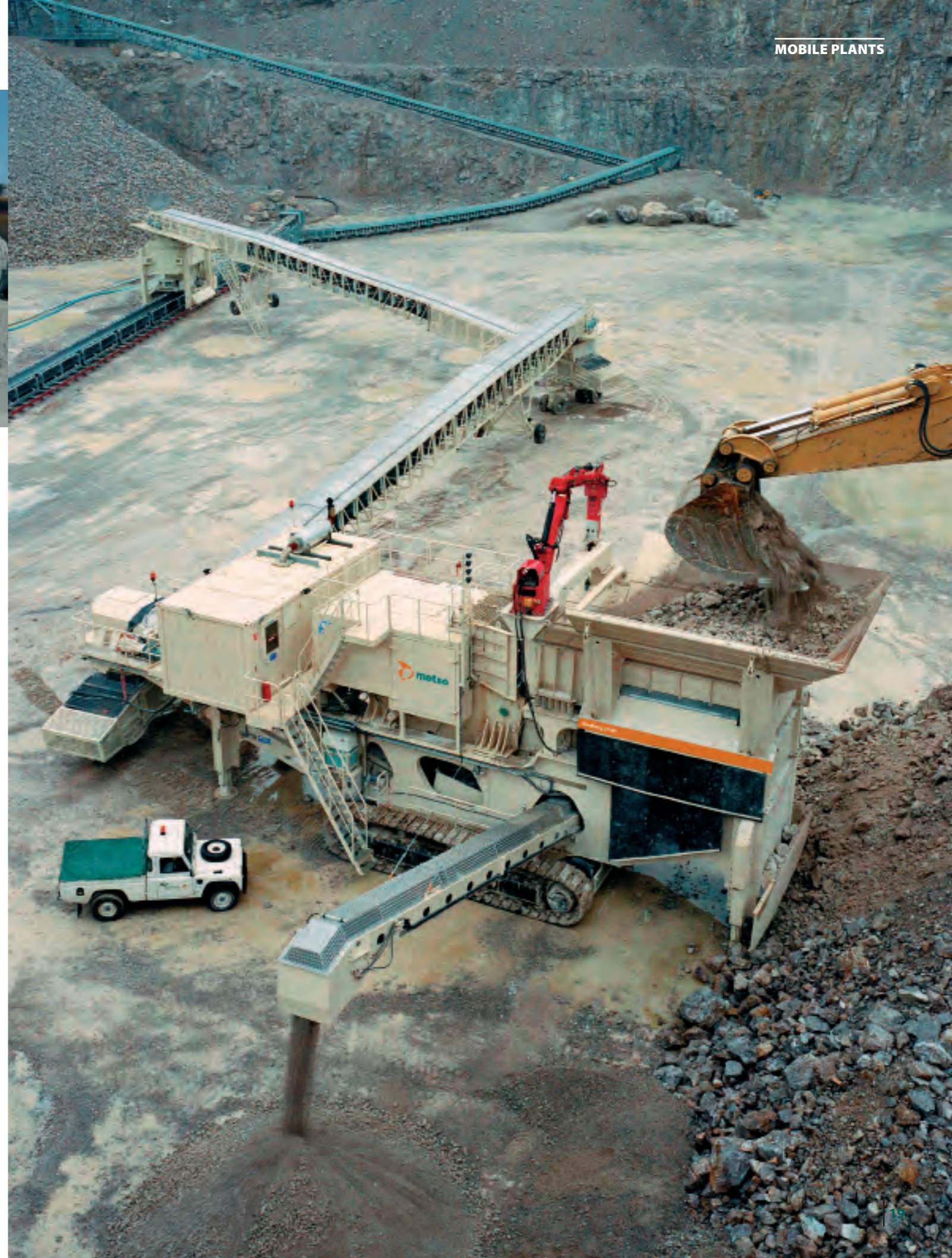
The gigantic Lokotrack LT160, coupled with Lokolink in-pit mobile conveyors, eliminates the need for haulage trucks.
