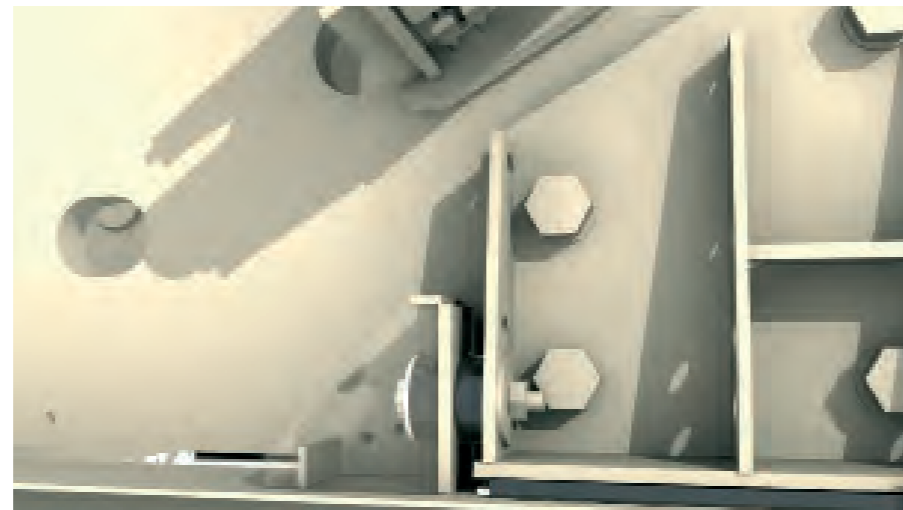
Special rubber dampers and stoppers allow the crusher to move vertically and longitudinally while preventing wear and subsequent damage to the crusher's foundation.
