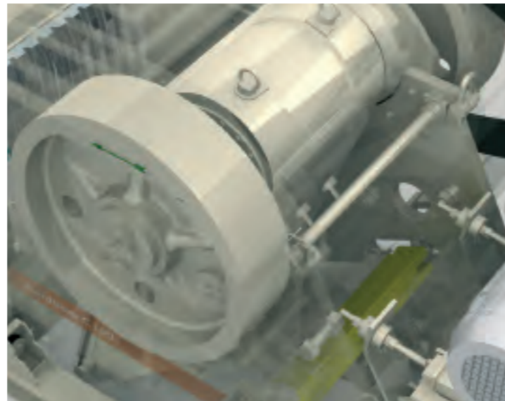
The robust pitman assembly ensures the greatest reliability even under the most severe crushing conditions.
