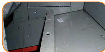
main belt - wear protection (only R1100)
